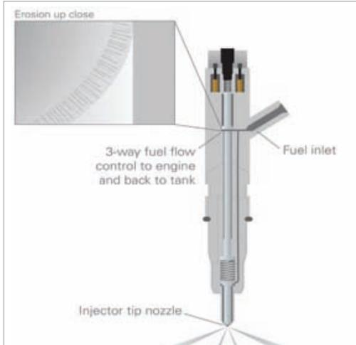
An example of the change in diesel injector patterns caused by wear from abrasive particles in dirty fuel.
