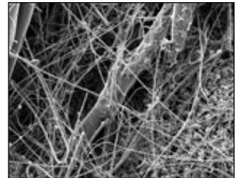
*Carboxylates under a scanning electron microscope at 500 times magnification.*
