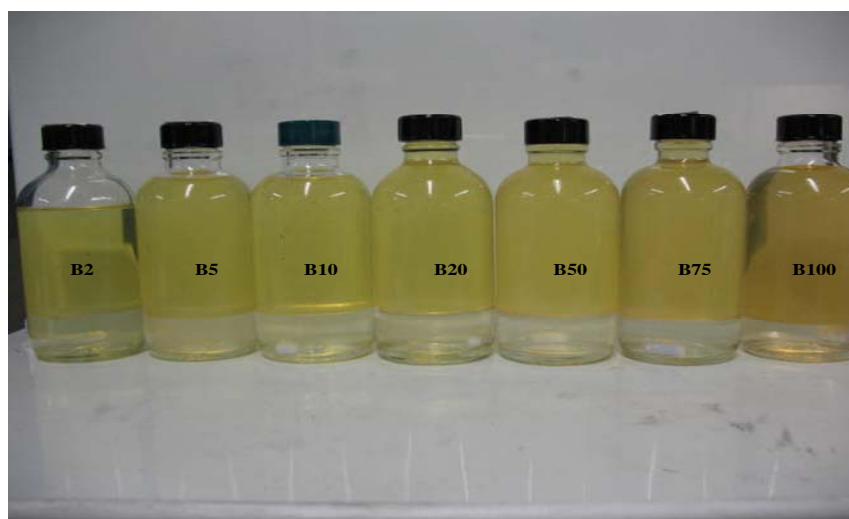
Fig.9 Color change of blended fuels saturated with water
