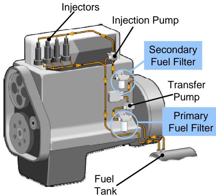
**Figure 12:** A typical fuel systems with both primary and secondary fuel filters
