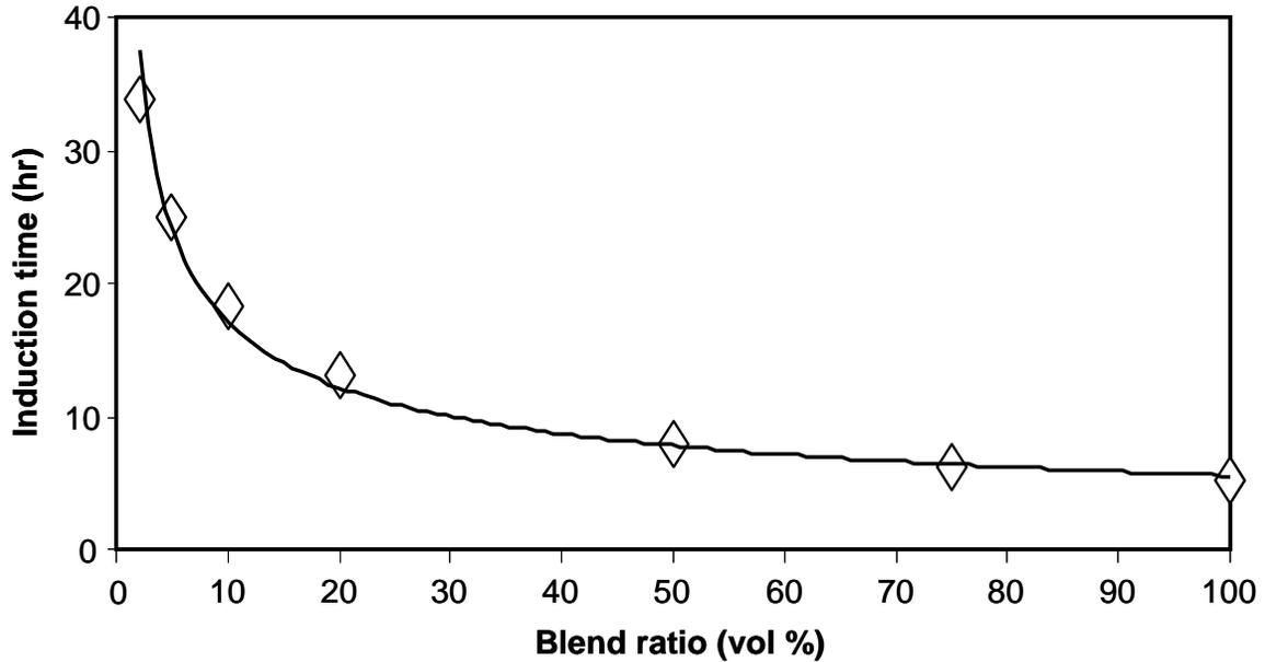
**Figure 8:** Induction time vs soybean biodiesel/ULSD blend ratio
