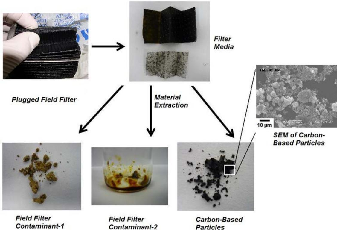
**Figure 7:** Field contaminants extracted from a plugged fuel filter.
