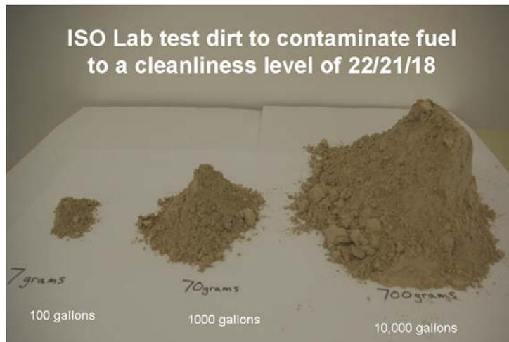
**Figure 16:** Amount of ISO medium lab test dust required to contaminate fuel to an ISO cleanliness of 22/21/18, or alternatively which must be filtered out of the given fuel volume.
