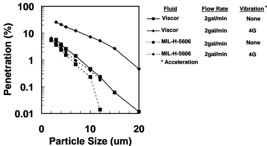
Figure 15: Effect of vibration on particle penetration
