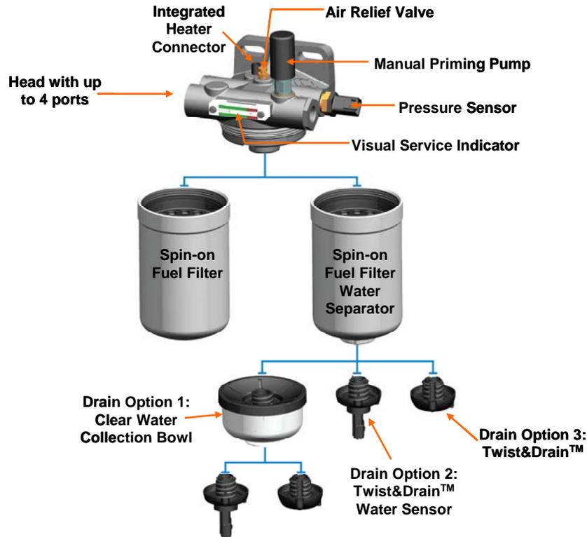
**Figure 11:** Remote mount fuel filtration assembly with optional features and functions
