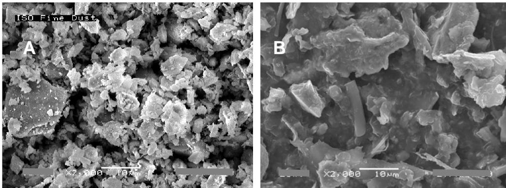
**Figure 3:** SEMs of: A) ISO fine dusts; B) a used diesel fuel filter
