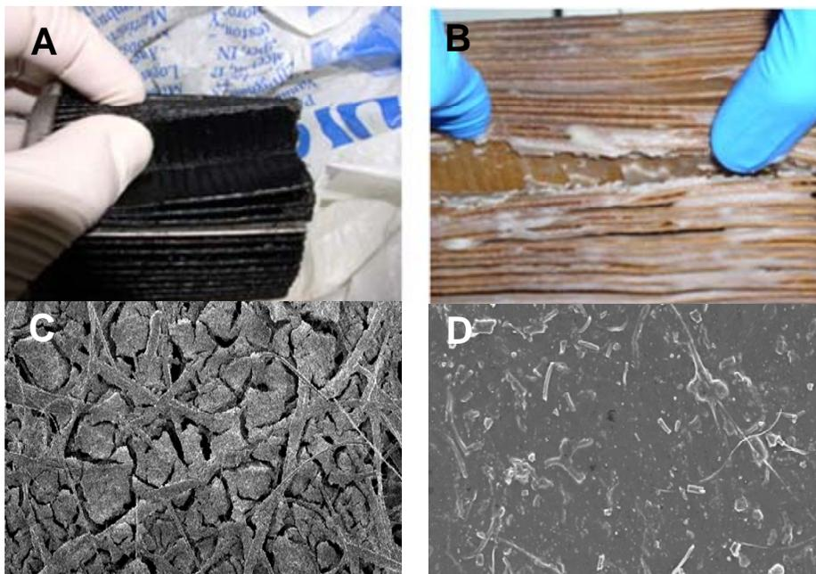
**Figure 6:** A) Plugged ULSD fuel filter, B) plugged biodiesel fuel filter, C) SEM of ULSD formed organic contaminants, and D) SEM of biodiesel formed organic contaminants
