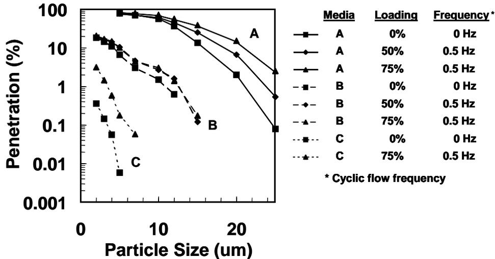
Figure 14: Effect of cyclic flow on particle penetration
