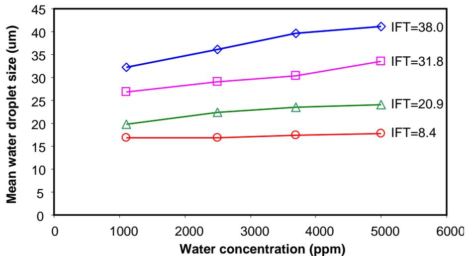
**Figure 5:** Mean droplet size as a function water concentration and IFT
