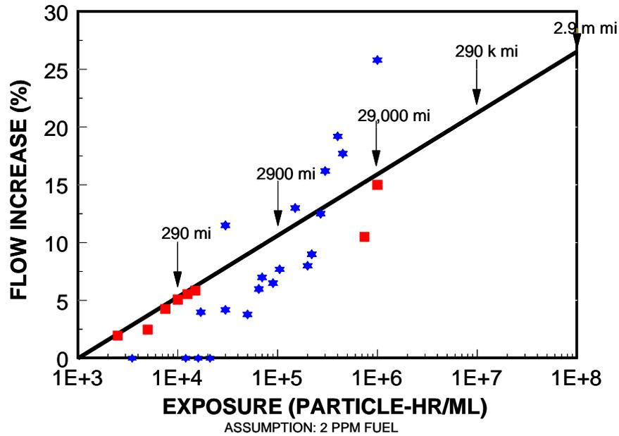
**Figure 2:** Fuel injector nozzle wear represented by increase in fuel flow as function of particle concentration
